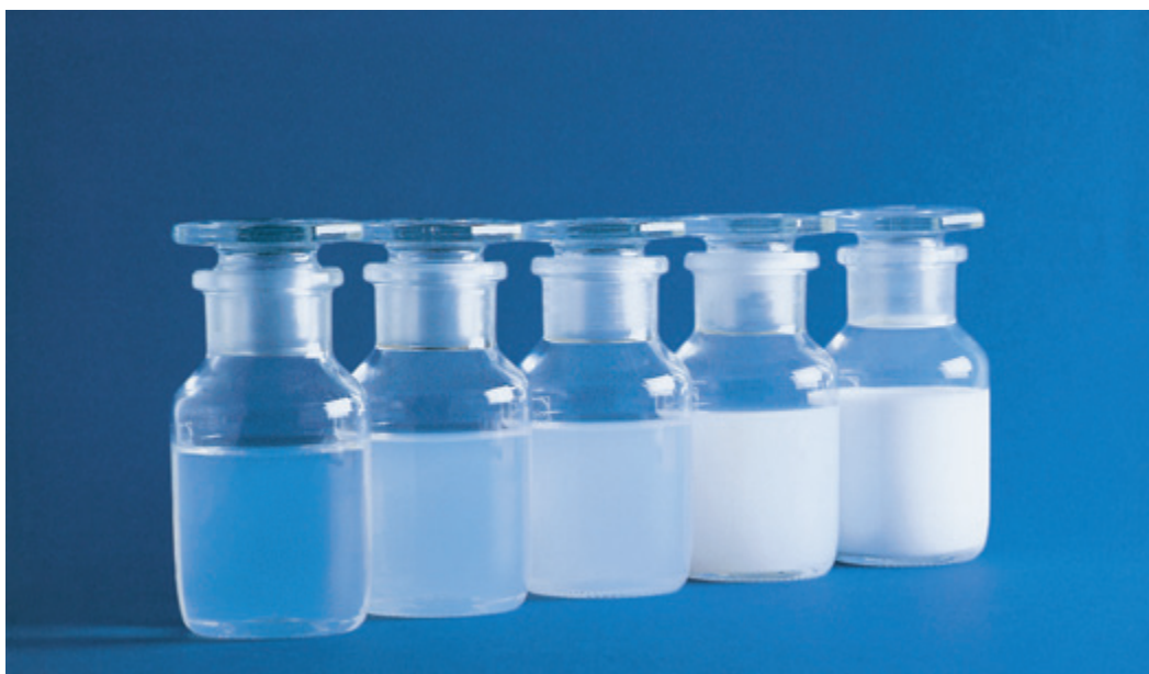
Figure 2: Translucent to opaque boehmite sols, each with a concentration of 10 wt.% \text{AlOOH}
